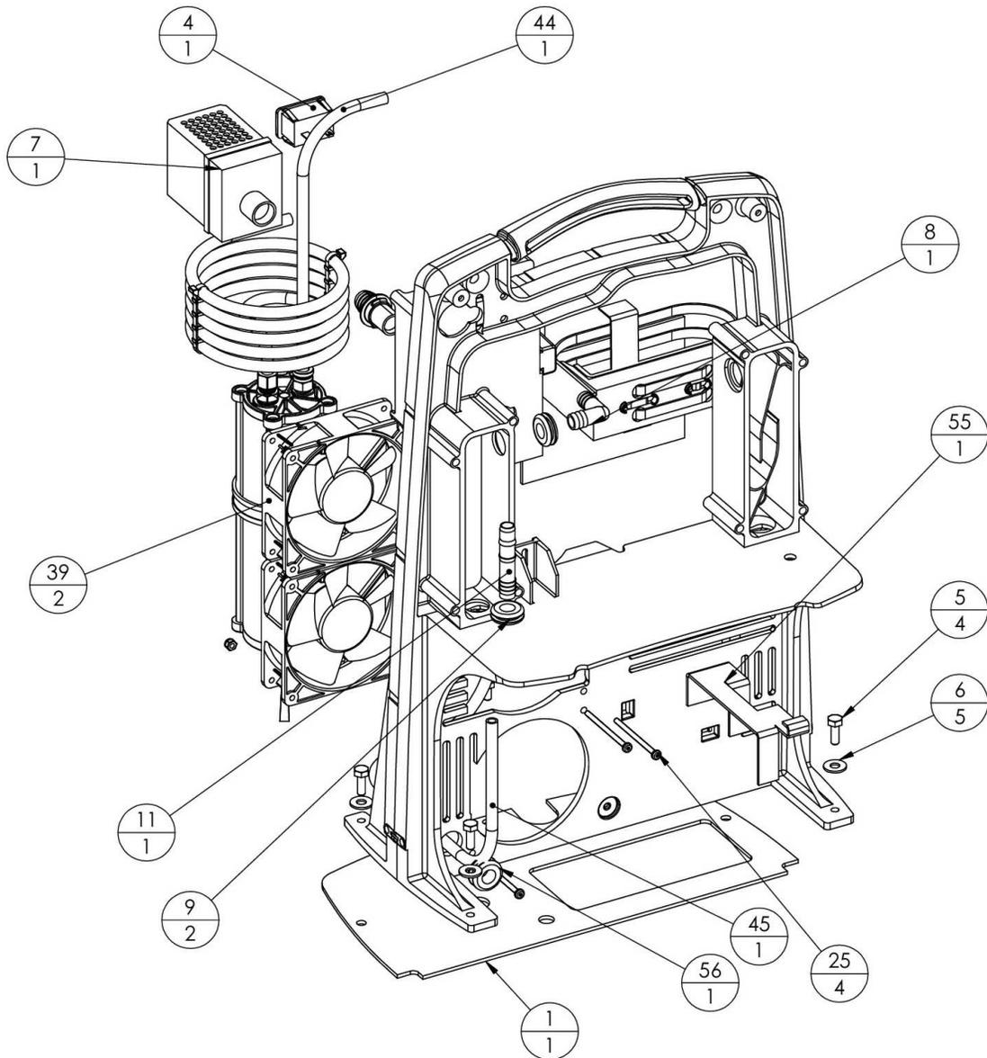
**A-4.4, Main Structure Assembly 10LPM unit**
