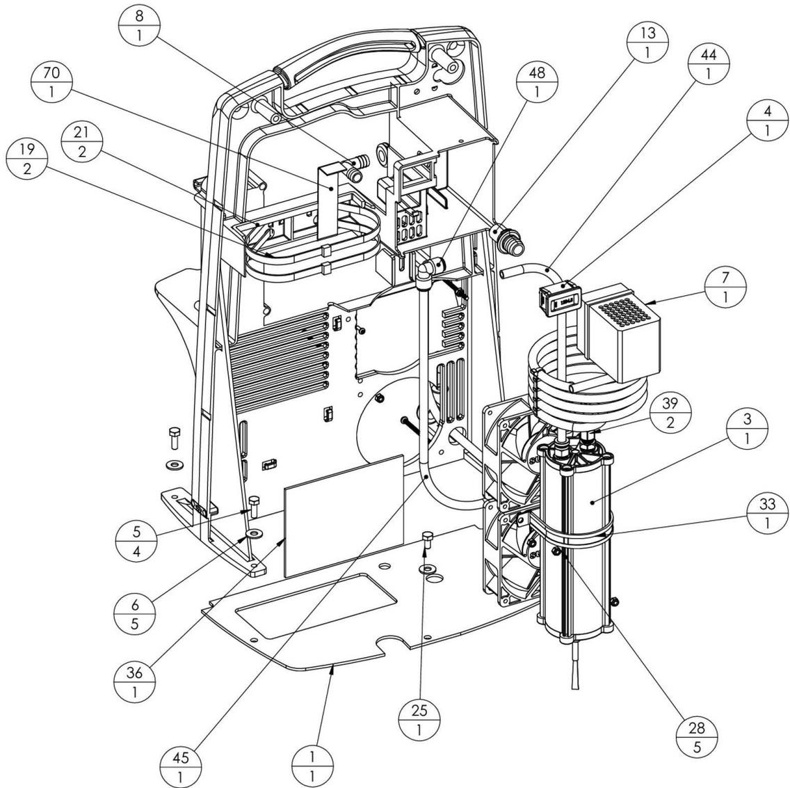
**A-4.5, Main Structure Assembly 10LPM unit**
