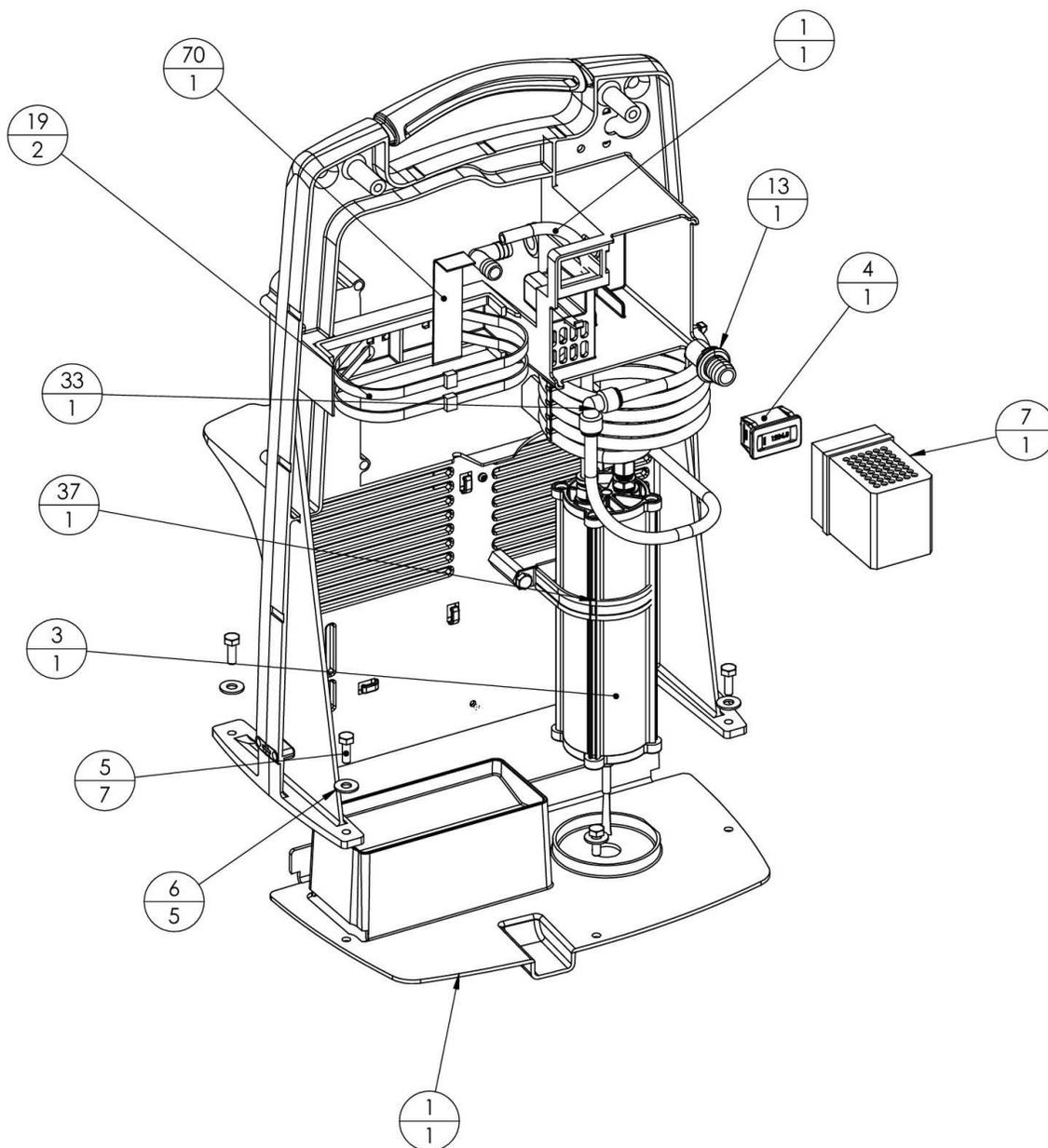
**A-4.1, Main Structure Assembly 5LPM unit**
